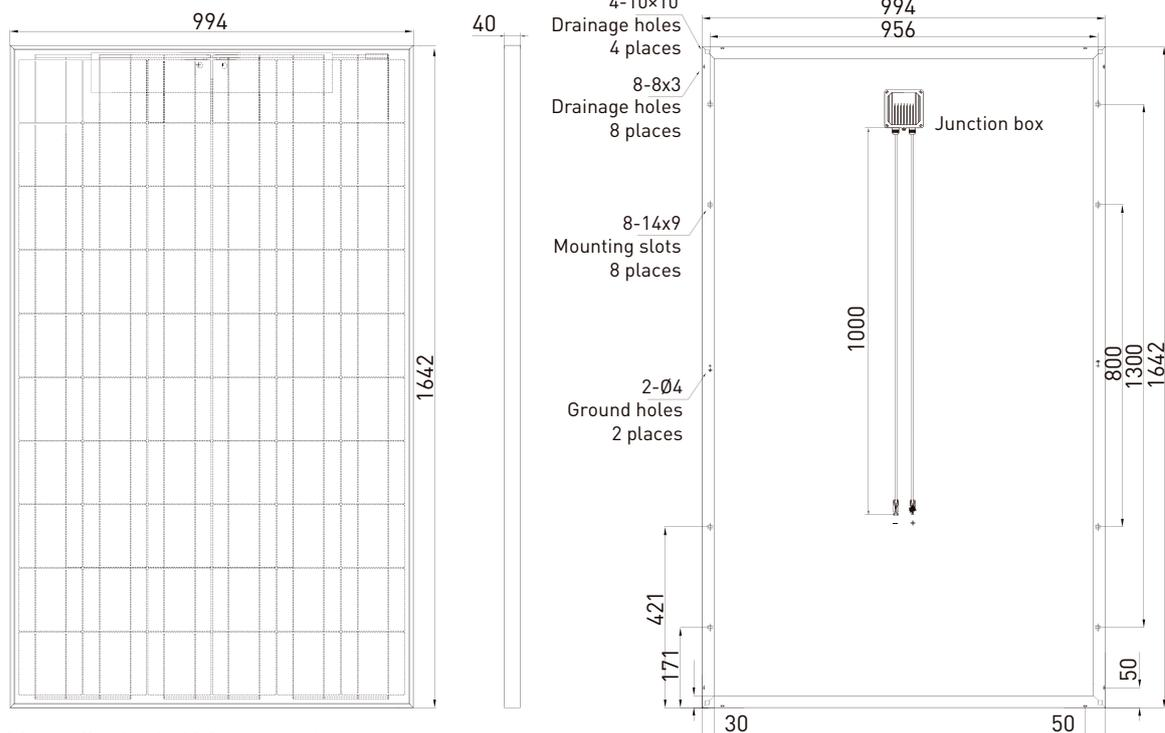
Tolerance of length and width dimensions is +/- 2 mm
