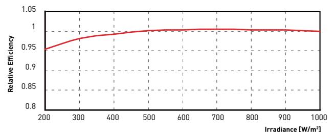
The typical relative change in module efficiency at an irradiance of 200W/m<sup>2</sup> in relation to 1000W/m<sup>2</sup> (both at 25 °C and AM 1.5 spectrum) is less than 6%
