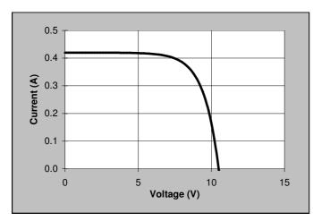
The electrical specifications are under test conditions of irradiance of 1 kW/m2, Spectrum of 1.5 air mass and cell temperature of  $25^{\circ}$ C. Minimum Power Output = Nominal Power - 10 %
