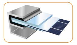
The special solar glass is highly transparent and has a self cleaning surface. As a result, dirt is reduced and the efficiency increases. The double-room profile makes the frame very strong and results in a perfect linking rigidity. The panel is snow resistant and can resist up to 35mm diameter hailstones as well as a 200kph wind.
