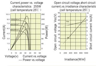
current, vs. irradiance characteristics (cell temperature:25°C )
