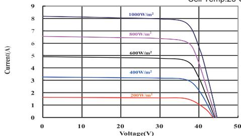
I-V Curves of CNPV-295PB at different cell temperature
