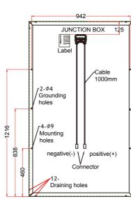
Dimension: 1676mm x 992mm x 40mm (46mm) Cells: 60 polycrystalline 156x156mm cells Connection: Junction box above IP65 with 3 bypass diodes Cable: 4mm<sup>2</sup> x 1.0m with Tyco or MC4 compatible connectors Frame: Anodized aluminum Weight: 40mm : 19 kg / 41.85 lbs 46mm : 20 kg / 44.05 lbs
