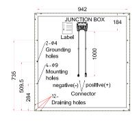
Dimension: 1019mm x 992mm x 40mm (46mm) Cells: 36 mono-crystalline 156x156mm cells Connection: Junction box IP65 with 3 bypass diodes Cable: 4mm<sup>2</sup>x1.0mm with Tyco or MC4 compatible
