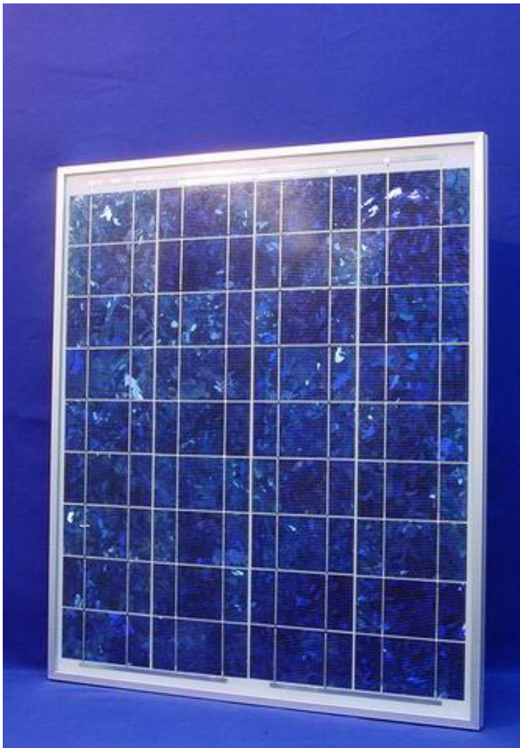
MG 25 : 25W, 12V, Poly-crystalline Si, Glass/EVA/Tedlar
