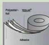
The improved gloss of the Tedlar surface effects a special reflection to the solar radiation to increase conversion efficiency and resist weather and moisture
