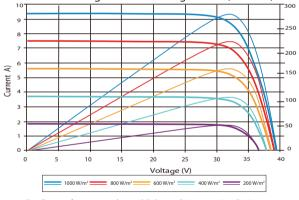
Current-Voltage & Power-Voltage Curve (280S-20)
