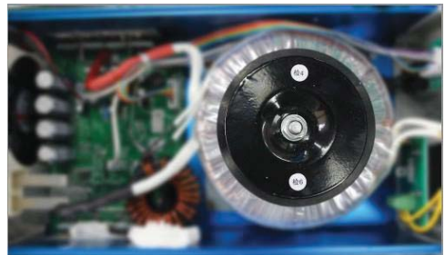
Big isolated transformer
